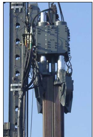
4 Cylinder Push-Pull Foundation Box Pile on Liebherr LRB255 - UK
